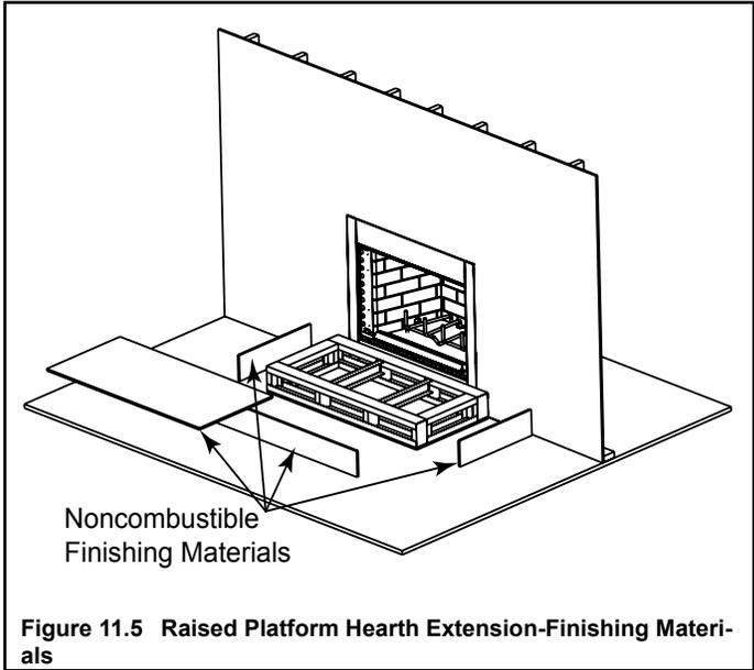
**Figure 11.5** Raised Platform Hearth Extension-Finishing Materials
