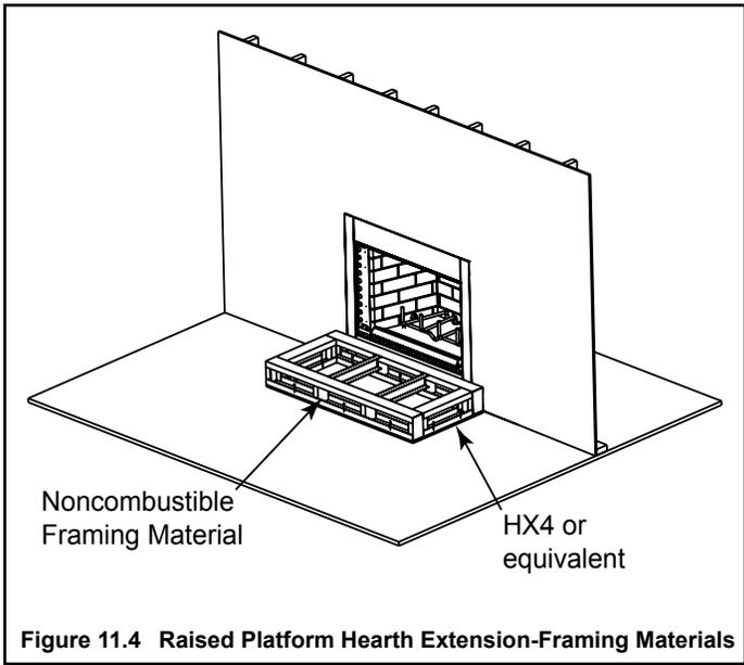
**Figure 11.4** Raised Platform Hearth Extension-Framing Materials
