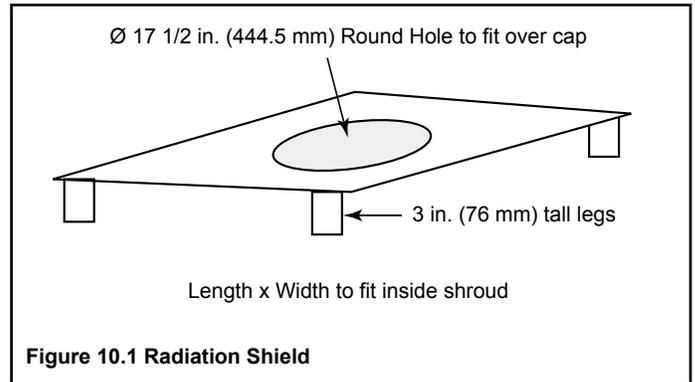
Figure 10.1 Radiation Shield
