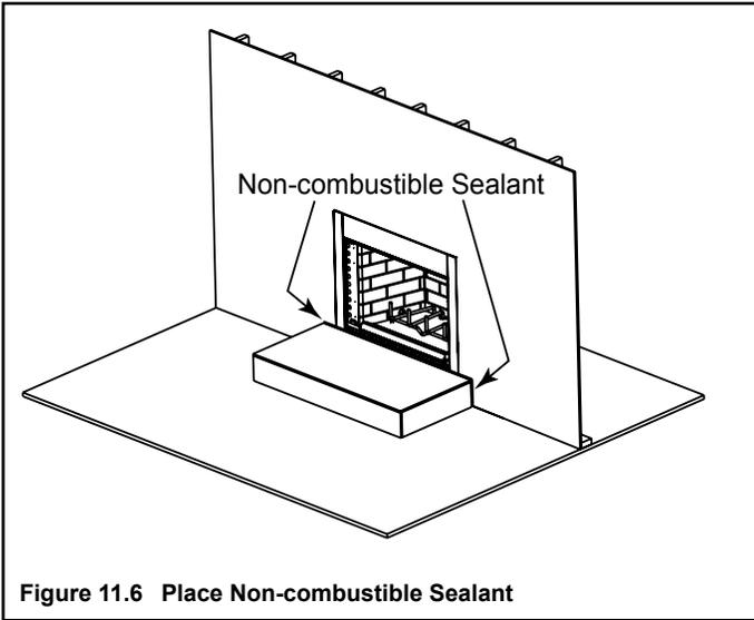
Figure 11.6 Place Non-combustible Sealant
