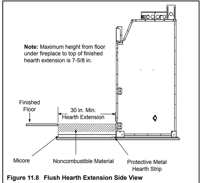
Figure 11.8 Flush Hearth Extension Side View
