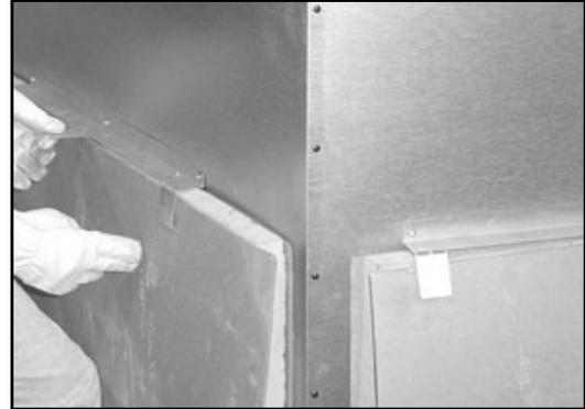
Figure 7.1 Unpacking Back Refractory
