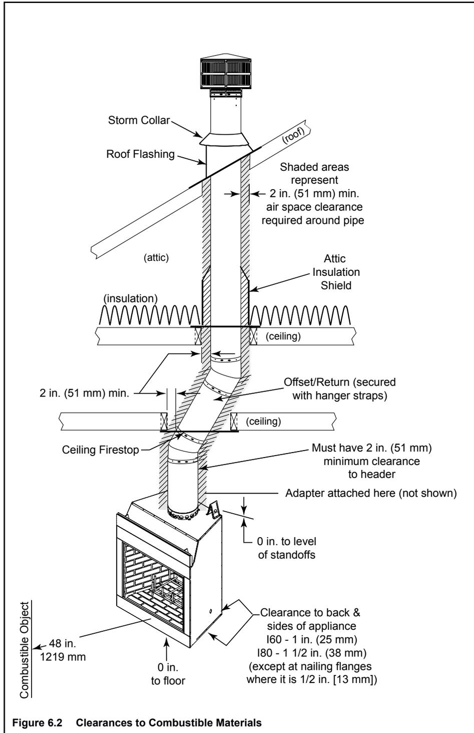
**Note:** Chimney air kit and 11-10 in./279-254 mm adapter are not shown, but are required in Canada.
