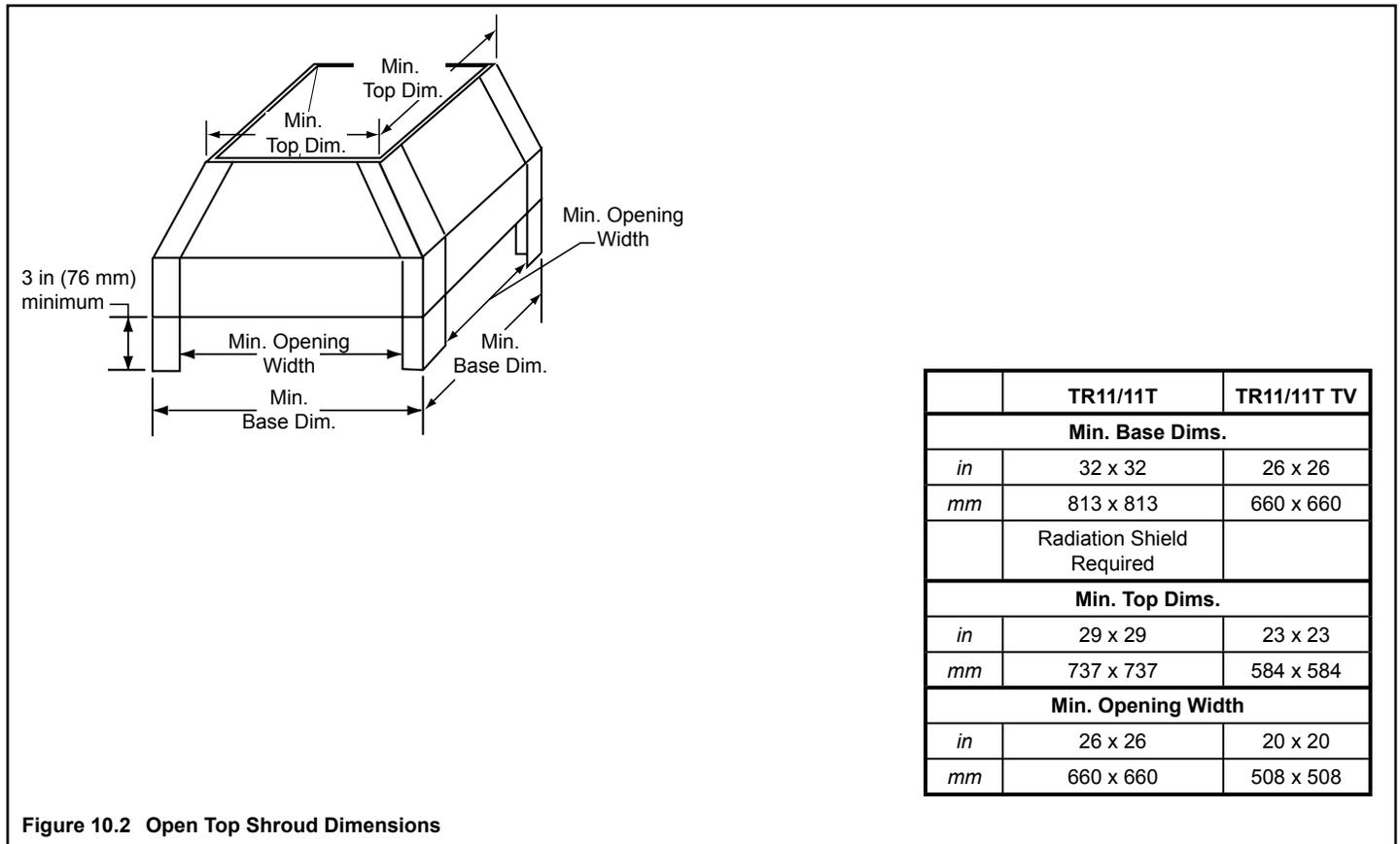
Figure 10.2 Open Top Shroud Dimensions
